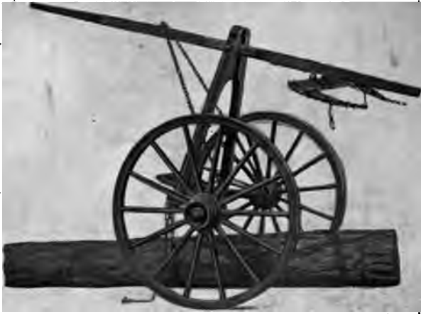
FIG. 45. — The Perry Log Cart in position to load. This cart has wheels either 4\frac{1}{2} or 5\frac{1}{2} feet high.
